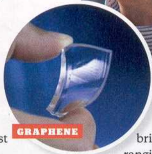
MODEL MATERIAL Physicist Andre Geim holds a model of graphene fibers. Inset: Actual piece of graphene, which is almost transparent.
